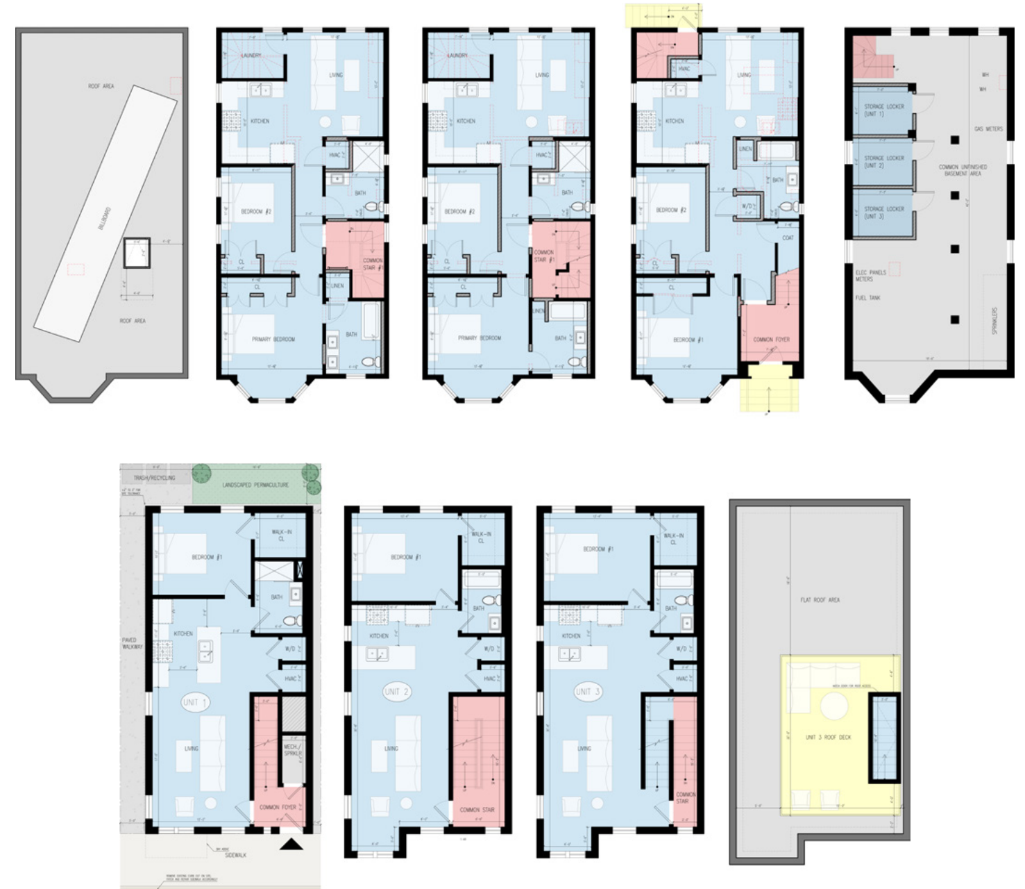
Above, top: A set of plans for an existing triple decker to be renovated but with shear walls kept in place to support the existing billboard on the roof. Above, bottom: A set of plans for a brand new triple decker. Both are on Paris Street in East Boston.
